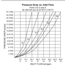
Flow vs. Differential Pressure FD50-45-X-X-44 (Dividing Mode)
