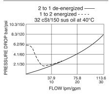
SV12-21 with Sensor 2 to 1 de-energized — 1 to 2 energized ----32 cSt/150 sus oil at 40°C 20.7/300 20.7/300 6.9/100 37.9 75.8 113.6 30 FLOW lom/gom
