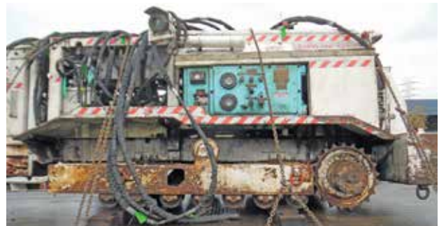
Condition of gas drainage drill rig prior to overhaul
