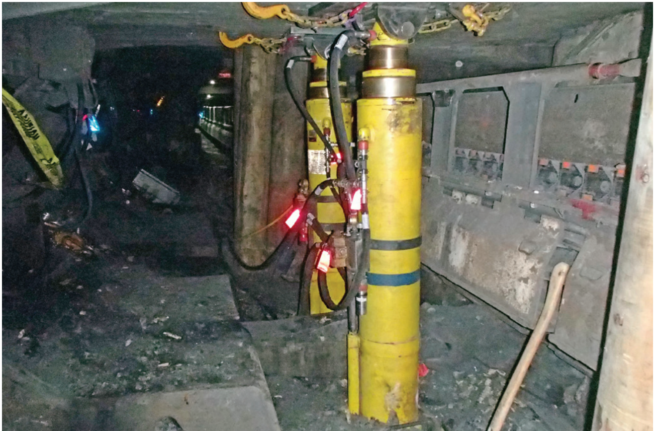
Bore support legs in use in longwall
