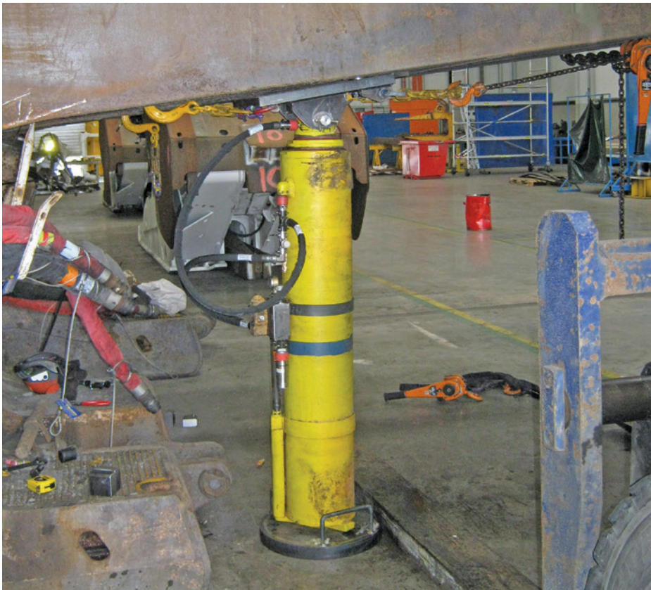
Bore support legs in Berendsen workshop
