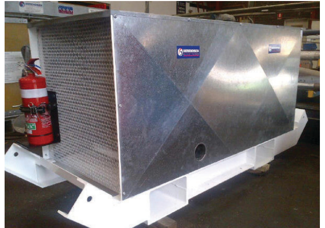
Completed diesel power unit ready for delivery
