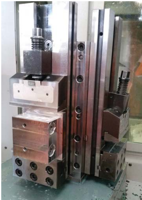
Manifold manufacture in progress using our CNC milling machinery at our Newcastle branch.
