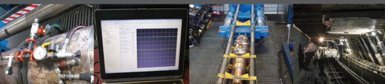
The testing of Roof Support Cylinders after repair is typically accomplished by restraining the leg within a frame and pressurising the leg to a predetermined test pressure. The flaw in this static method of testing is that it does not provide a true simulation of the forces that the cylinder is exposed to under normal working conditions.
