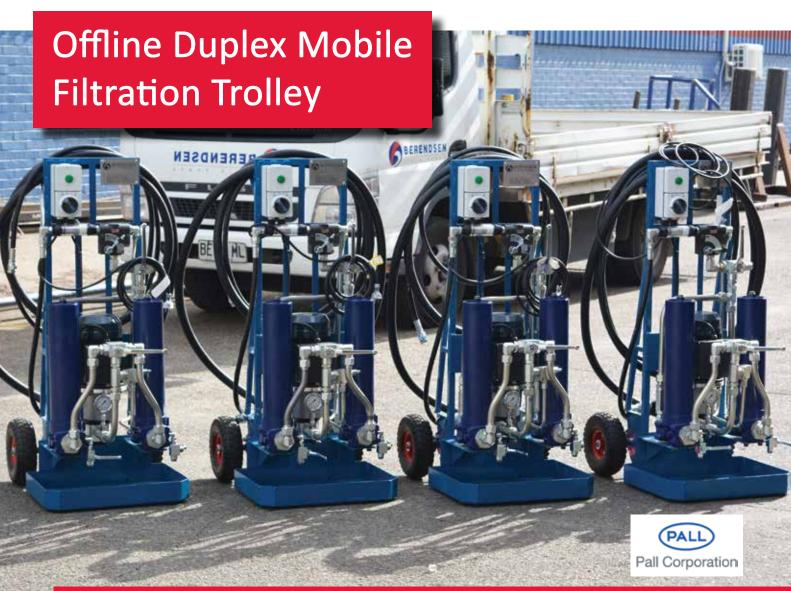
Berendsen Fluid Power's Offline Duplex Mobile Filtration Trolley is used to clean/filter a wide range of industrial fluids on the go. The duplex filter set up enables constant filtering even when the element reaches its end of life.
